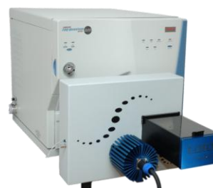
Figure 2: LDTD system on Thermo Vantage Mass Spectrometer.
