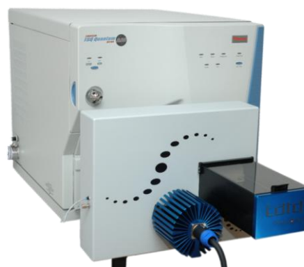
Figure 2: LDTD system on Thermo Vantage Mass Spectrometer.
