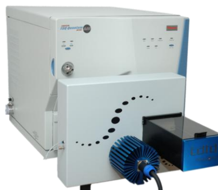
Figure 2: LDTD system on Thermo Vantage Mass Spectrometer.
