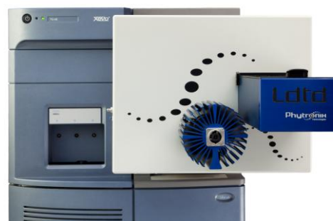
Figure 2: LDTD system on Xevo-TQMS mass spectrometer
