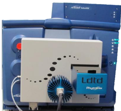
Figure 1: LDTD system on AB SCIEX 5500 Qtrap Mass Spectrometer
