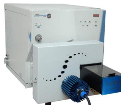
Figure 2: LDTD system on Thermo Vantage Mass Spectrometer
