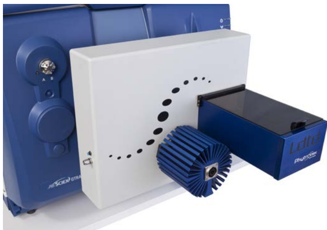
Figure 1: LDTD system on AB SCIEX 5500 Qtrap Mass Spectrometer
