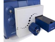
Figure 2 LDTD system on Sciex 5500 QTrap<sup>®</sup>
