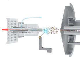
Figure 2 Schematic of the LDTD ionization source
