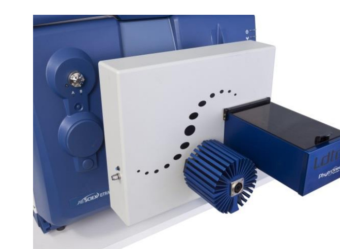
Figure 3 LDTD ® model S-960 coupled with Sciex QTRAP ® 5500
